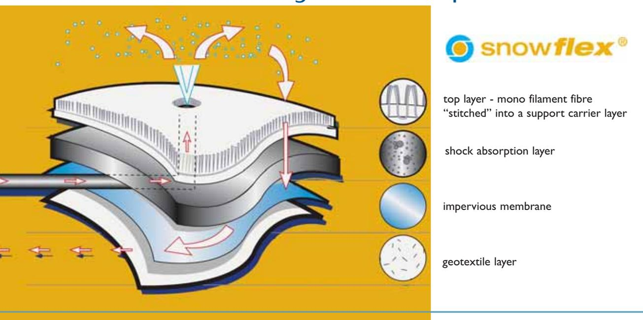
Snowflex® is a homogeneous polymer composite with a high-tech meltless sliding layer suspended over a shock-absorption layer. It is manufactured on a production line specially designed and developed by Briton Engineering in Yorkshire, England.
